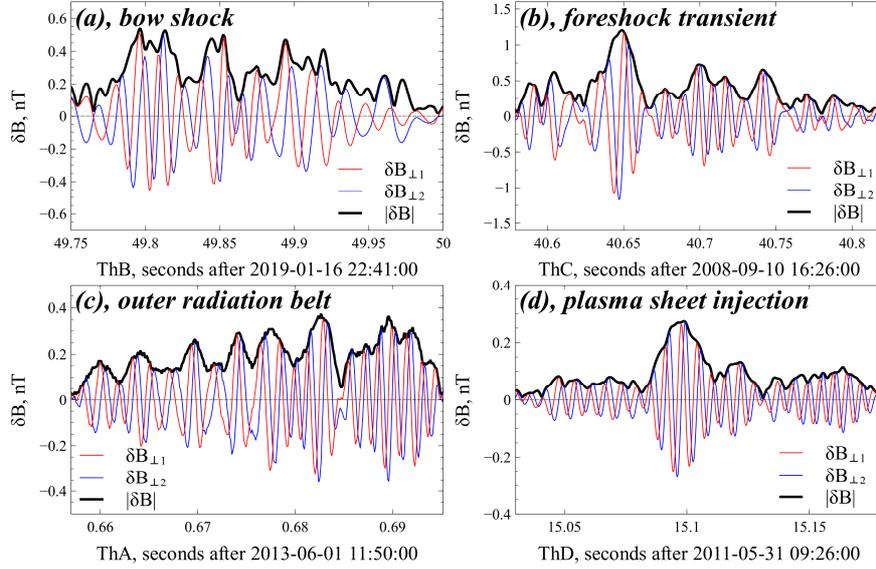
Figure 1. Examples of typical wave-packets of whistler-mode waves captured by THEMIS spacecraft [Angelopoulos, 2008] in Earth bow shock (a), foreshock transient (b), outer radiation belt (c), plasma injection region (d). These events are picked up from statistics published in [Artemyev et al., 2022; Shi et al., 2020; Zhang et al., 2018b, a]
