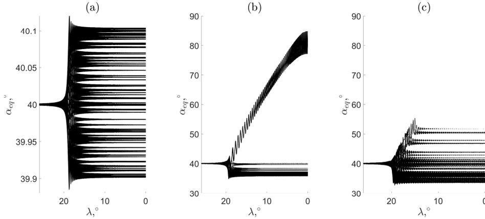
Figure 2. Set of trajectories for low amplitude wave with diffusive scattering (a), coherent high-amplitude wave with trapping and bunching (b), modulated high-amplitude wave with diffusive-like scattering (c). System parameters are: electron energy  $E_0=100$  keV, equatorial pitch-angle  $\alpha_0=40^\circ$ , number of particles  $N=100$ , wave amplitude  $B_w=5$  pT (a),  $B_w=500$  pT (b, c)
