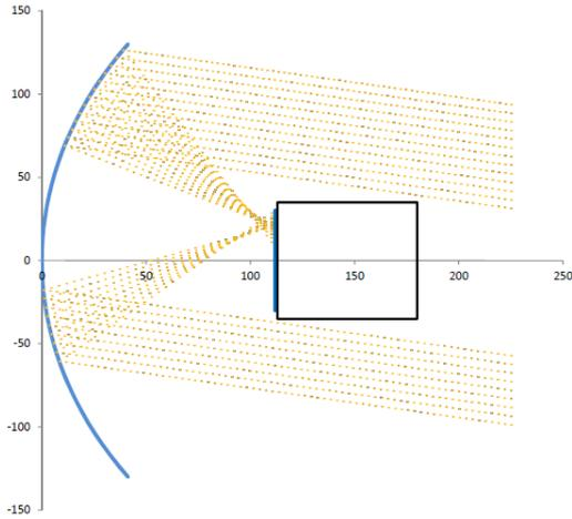
Fig. 1. Modeling rays (yellow points) from a distant point source in the telescope. Blue curves illustrate the mirror and photocathode surface. Black rectangle imitates shadowing by the PMT case.
