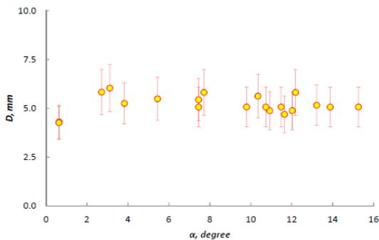
Fig. 3. Fuzzy image diameter of the distant point source on the photocathode surface as a function of incidence angle,  $\alpha$ .
