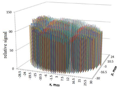
Fig. 5. Normalized coordinate-dependent sensitivity of the photomultiplier.
