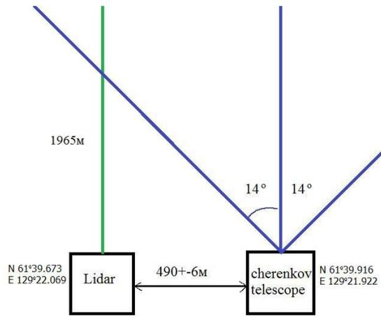
Fig. 6. LIDAR signal entering into the aperture of the telescope flowchart.
