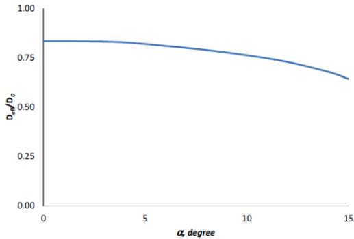
Fig. 2. Shadowing of the mirror by the PMT and support + cables. The ratio of unshielded effective mirror diameter to the actual diameter is given as a function of incidence angle,  $\alpha$ .
