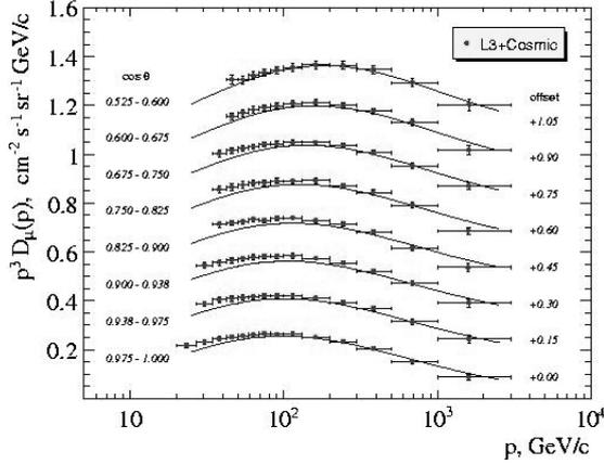
Fig. 4. Calculated atmospheric muon energy spectrum and recent results of L3+Cosmic experiment for zenith angles 0–58°. Calculations are performed for the ATIC-2 primary cosmic ray spectra. Solid curves correspond to the average zenith angles for given angle bin.
