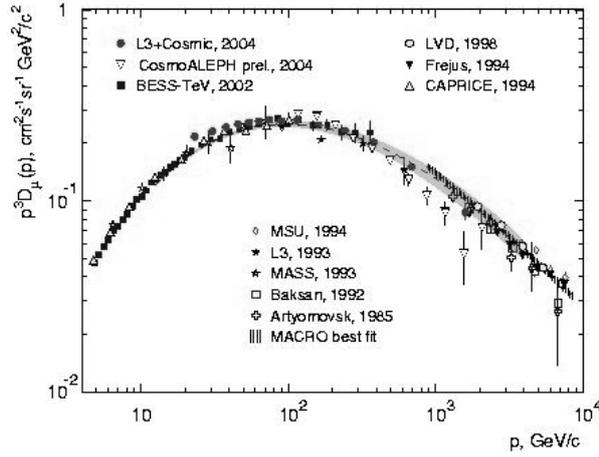
Fig. 2. Energy spectrum of muons at ground level near vertical. The dashed-line curves and the shaded area present this work calculation with the ATIC-2 primary cosmic-ray spectrum.
