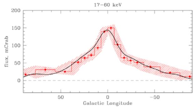
*Fig. 1.* Longitude profile of the GRXE measured by INTEGRAL/IBIS/ISGRI (histogram and shaded region) in the 17–60 keV energy band along with the intensity profile of the Galactic NIR emission obtained by COBE/DIRBE at 4.9  $\mu$ m (solid line). The NIR map was convolved with the IBIS collimator response.
